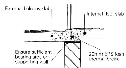
Balconies extended from the main slab of a house may act as cooling or heating fins, carrying precious warmth away to the cold exterior during winter, or transferring heat from summer sun inside. Consider building such slabs independently of the main slab and incorporating a thermal break at the interface.
