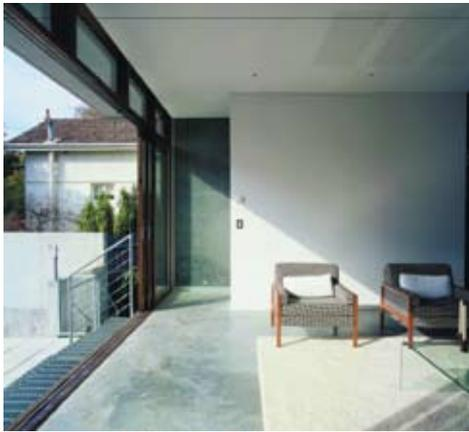
Thermal Mass describes the potential of a material to store and re-release thermal energy. Materials with high thermal mass, such as concrete slabs or heavyweight walls, can help regulate indoor comfort by radiating or absorbing heat, creating a heating or cooling effect. [See: 4.9 Thermal Mass]
