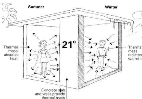
Design slabs to absorb heat from the sun or other sources during winter. Heat can be stored in the slab and re-radiated for many hours afterwards. In summer, allow slabs to be exposed to cooling night breezes so that heat collected during the day can dissipate.
