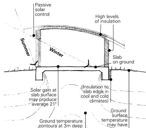
Earth coupling allows the floor slab of a well insulated house to achieve the same temperature as the earth a few metres below the ground surface, where temperatures are more stable (cooler in summer, warmer in winter). In winter, added solar gain boosts the surface temperature of the slab to a very comfortable level.
