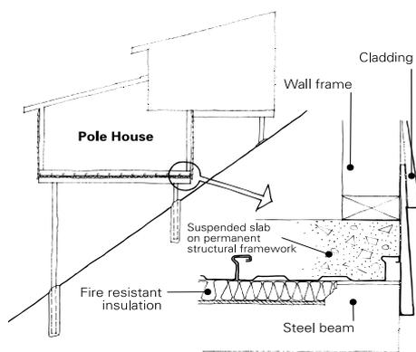
Permanent structural formwork or one of the many precast flooring alternatives are usually the most cost effective way of constructing high set suspended slabs. These are normally designed by an engineer and installed by builders.
