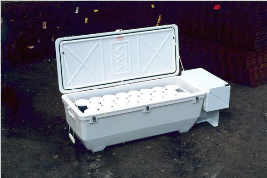
An example of proper field curing methods includes the use of a temperature controlled curing box
